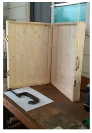
The two open-faced halves were then attached with hinges, latches and a handle to create a suitcase-style box.
