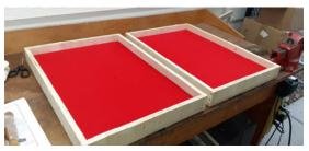
The case was then stained, and standoffs attached to the back pieces to mate with the pegboard standoffs.
