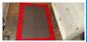
the pegboard panels to the back of the case halves, leaving a gap to accommodate the ties that would hold the tools in place and allowing for the pegboard panels to be removed if needed.
